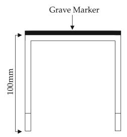
2x Horizontal Drilled & Countersunk Holes for Painted Security Screws
